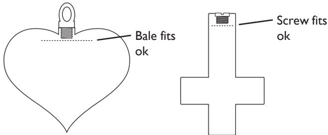
Place the screw all the way in the pendant with no glue applied yet. Make sure the threads are matching up well. Do not force the bale or screw closed. If the screw doesn't go in all the way, the piece may be overfilled.
