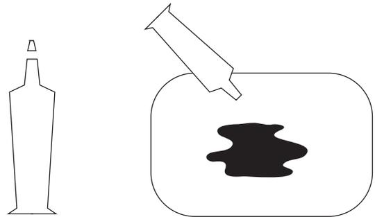
Cut a small opening at the top of the tube of glue. Squeeze some glue out on to a piece of paper or cardboard (enough to create a small puddle that you can dip the toothpick in to).
